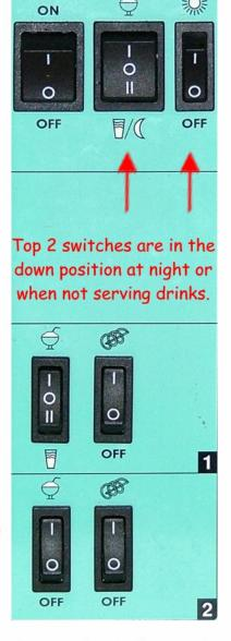
Bottom 4 switches are in the up position at all times.
