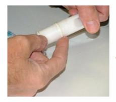
Put about 1/2" of grease on finger and apply on top of o-ring.
